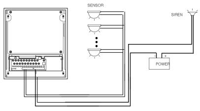
**Sensor In**: Connect the sensors. The sensor are composed of both signal and ground terminals, with a voltage difference of 5V. In the case that the sensor used for input is of the N/O (Normal Open) type, when the voltage difference between the signal and ground falls to 0V (short), the DVR can use this as a trigger to start alarm/sensor based recording.
