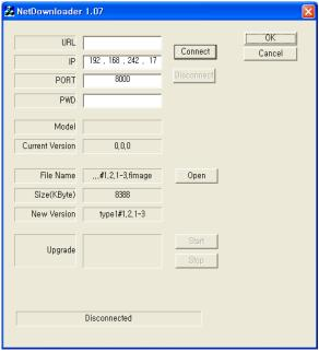
After typing the IP and password of the DVR, click the 'Connect' button. You can check the model name and the current version. If you can't see the model name and current version, you should check the network and try again.
