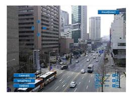
• Setup: If you press Setup using mouse (or Menu button on the remote controller) in PTZ Menu, PTZ setup window will appear. You can set the pan and tilt speed, 32 preset name and tour sequence as well as dwelling time,
